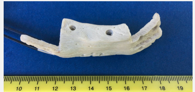
Figure 3 | Example of a PEKK bone analog manufactured using FDM (Chang et al., 2020)
